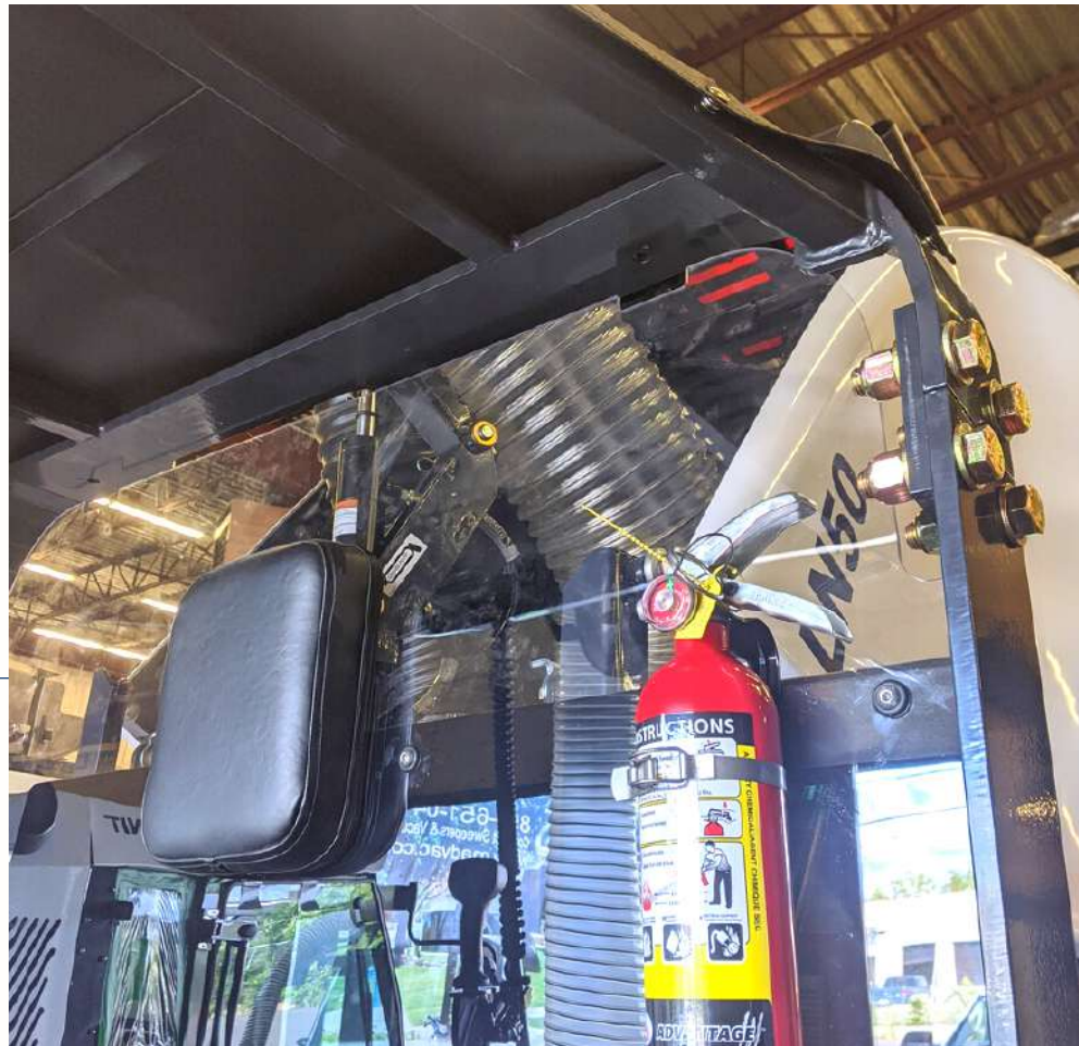
R.O.P.S. rollover protection system
