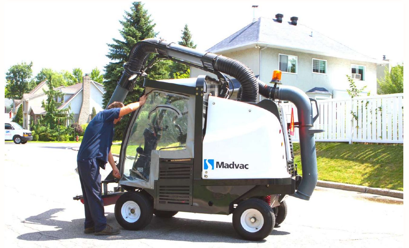
Enclosed cab with heated or non-heated windshield and vinyl doors
