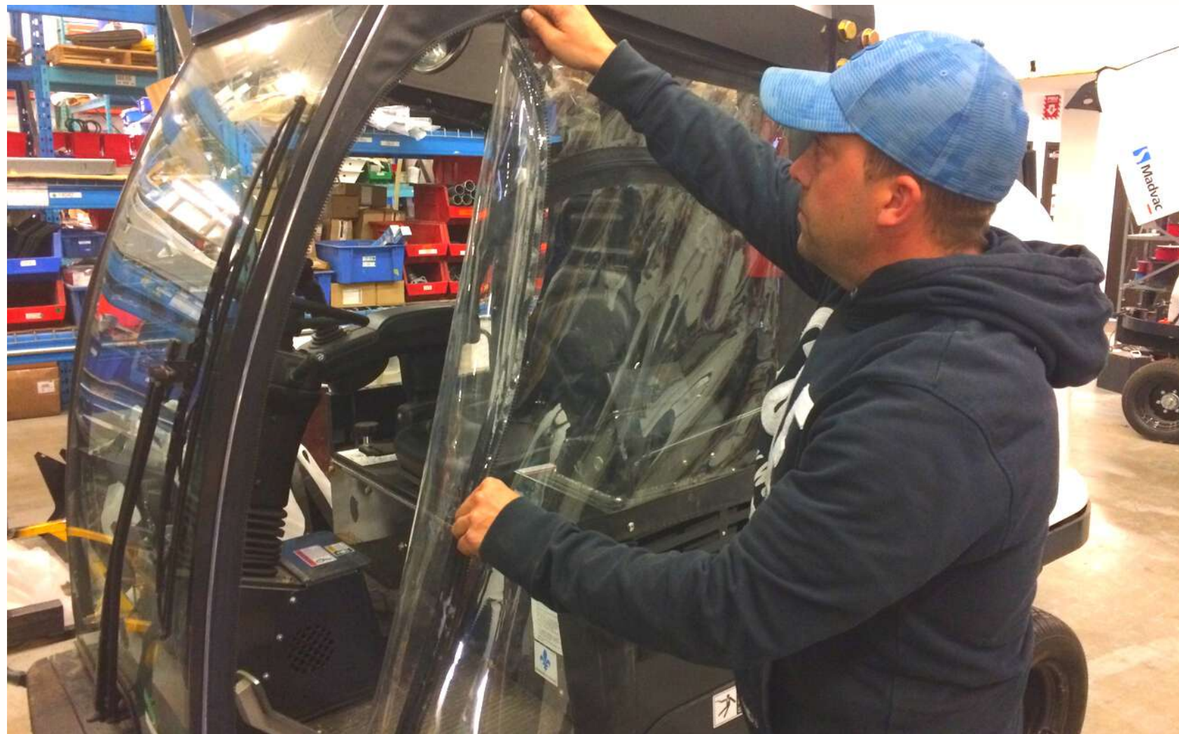
Enclosed cab with heated or non-heated windshield and vinyl doors
