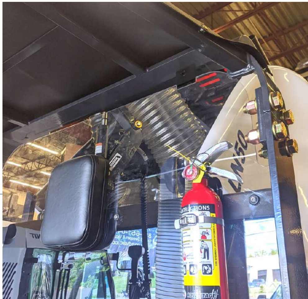
R.O.P.S. rollover protection system
