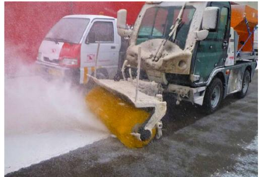
Snow broom | 59" (1500 mm) with hydraulic lifting plate
