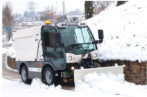
Snowplow | blade 59" (1500 mm) | hydraulic swivel | with attachment plate
