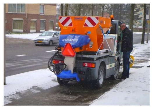
Salt spreader | hydraulic powered | capacity 1.7 cu yd. (1.3 m<sup>3</sup>)
