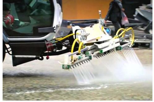
Street washer | plastic water tank capacity 528 gal. (2000 L) | 3 section swivelling telescopic spraying bar | width from 51" to 98" (1300 to 2500 mm)
