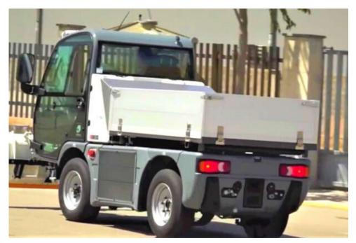
Aluminium cargo bed with trilateral tipping (left, right, rear) | 72.5" x 51.2" x 16.5" (1840 x 1300 x 420 mm)
