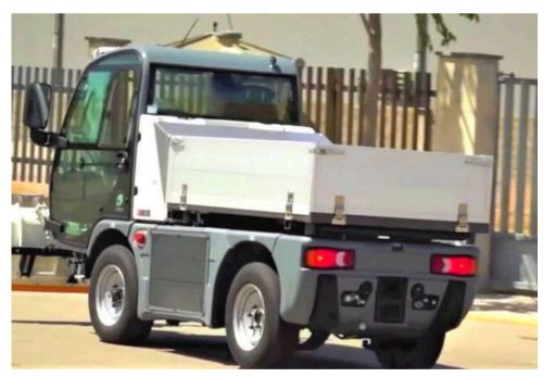
Aluminium cargo bed with fold down sides and hydraulic trilateral (rear/side) dump 72.5" x 51.2" x 16.5" (1840 x 1300 x 420 mm)
