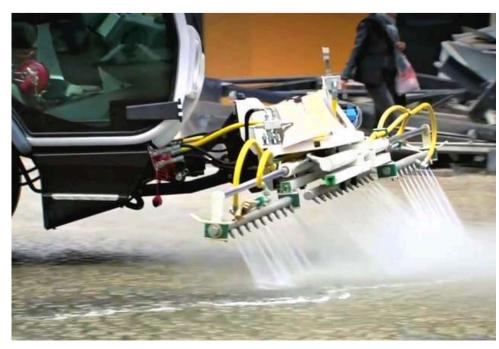
Cold water street-washer spray bar | Joystick controlled (3-stage swiveling/telescopic) Rotomold plastic water tank | capacity 528 gal. (2000 L)
