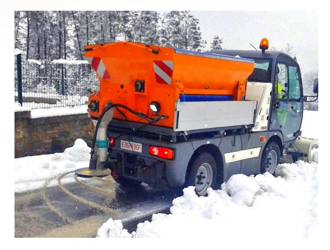
Salt spreader | hydraulic powered | capacity 1.3 cu yd. (1 m³)
